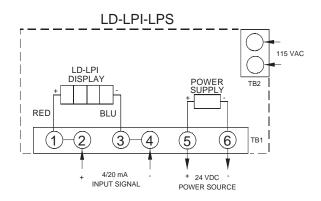
Fig. 1 Internal Wiring of LD-LPI-LPS
