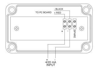
Fig. 5 Field Wiring
